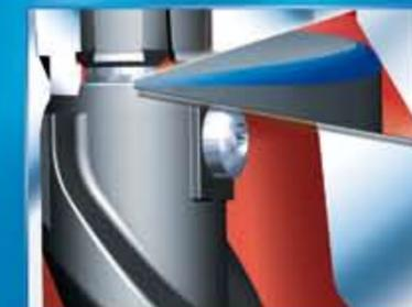
5. Back sealing of the plug provides added safety
